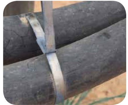
Image shows blue coating fading from stainless steel cable tie.
